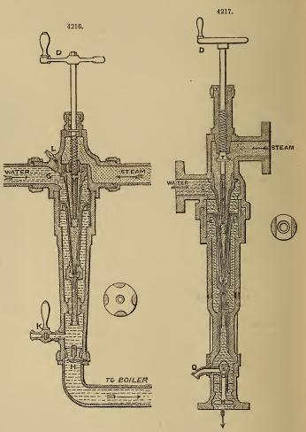
valve S, and stops the escape through the waste-pipe. This arrangement has the advantage not only of rendering unnecessary the opening and closing by hand of the waste-cock, but also of showing very clearly when the injector ceases working; because when that happens the boiler-valve H is closed by the back pressure from the boiler, opening simultaneously the valve S and allowing the steam and water to escape through the waste-pipe Q.
